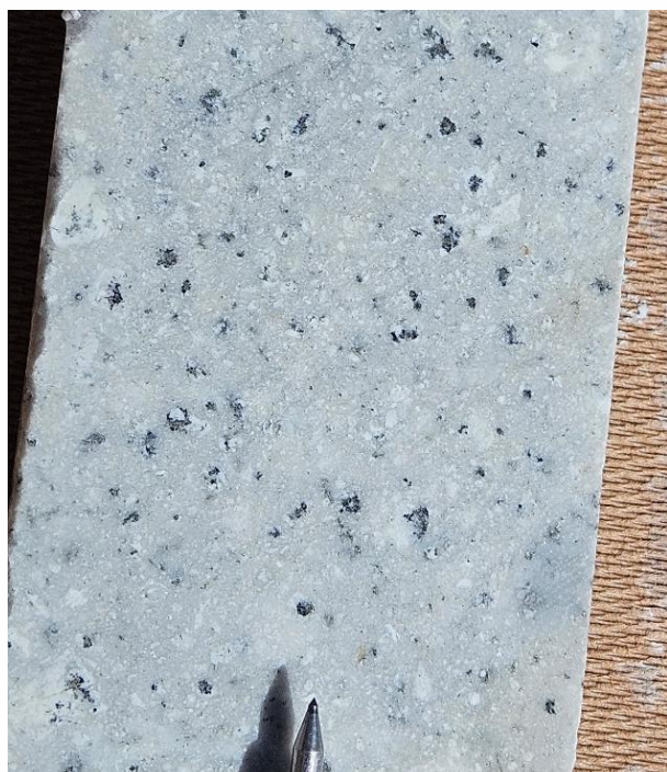
Figure 3: Core photo from Tambo South drill hole TMT-TSU-DDH-002 at 319m depth, showing a medium-grained, grey dioritic porphyry. Strong quartz-sericite (phyllic) alteration partially destroys the original texture. In the 248m to 375m interval, the visual estimate 1 of covellite, associated with pyrite, typically ranges from 0.2–0.6 volume-%, and locally reaches up to 1.0 volume-%.
