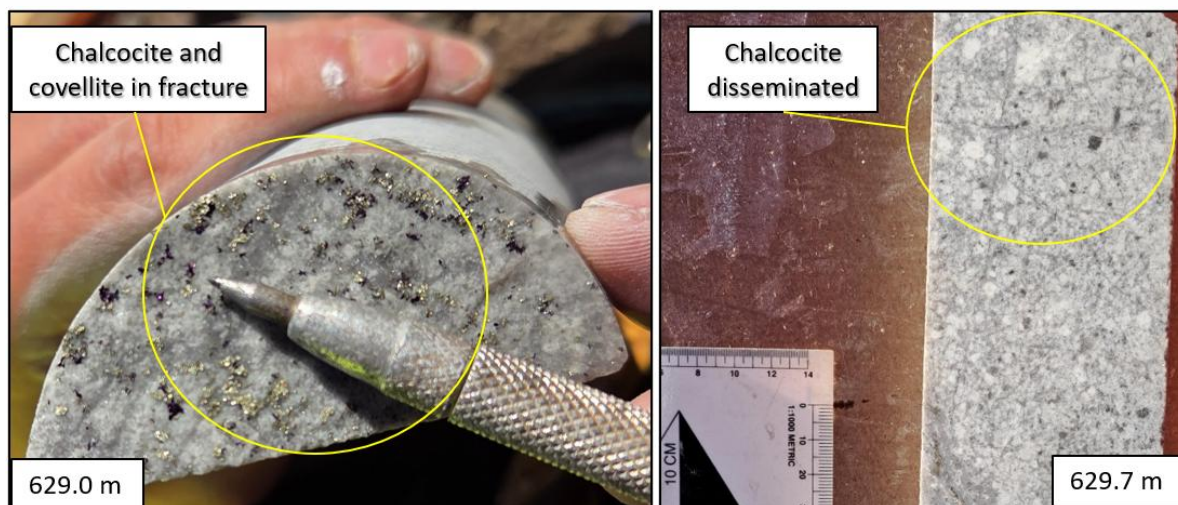
Figure 4: Core photo from Tambo South drill hole TMT-TSU-DDH-002 at 629m depth, showing a medium-grained, grey dioritic porphyry. Disseminated Py (3.0 volume-%), chalcocite (0.6 volume-%), and covellite (0.3 volume-%) are observed in the 2m-interval (629m to 631m) that contains these drill-core samples.
