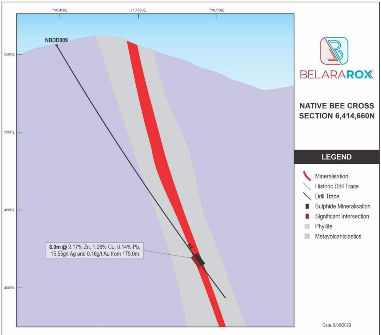
Figure 4. Cross section looking north at Native Bee showing drill intersection from NBDD009.
