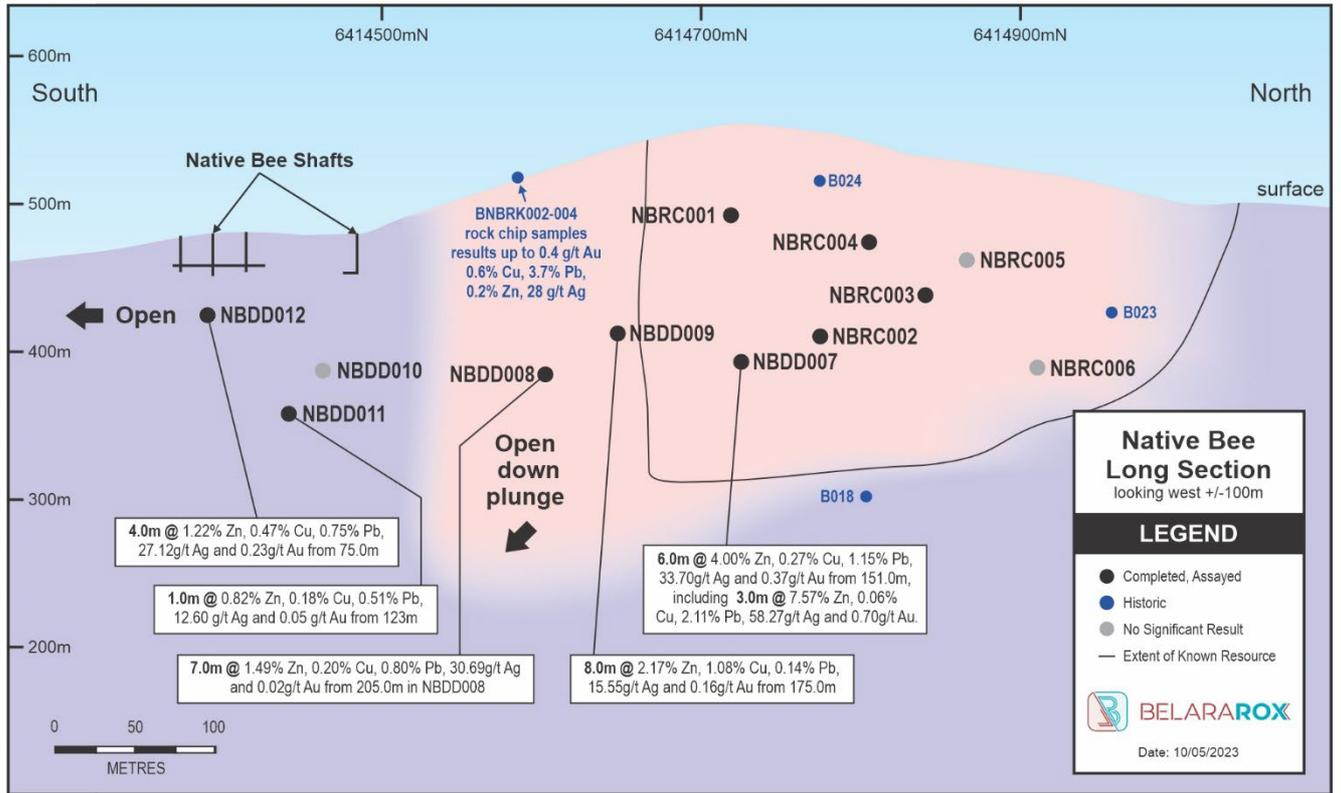
Figure 2. Long section at Native Bee showing drill intersections from Phase 2 drilling. Note that mineralisation remains open down plunge.
