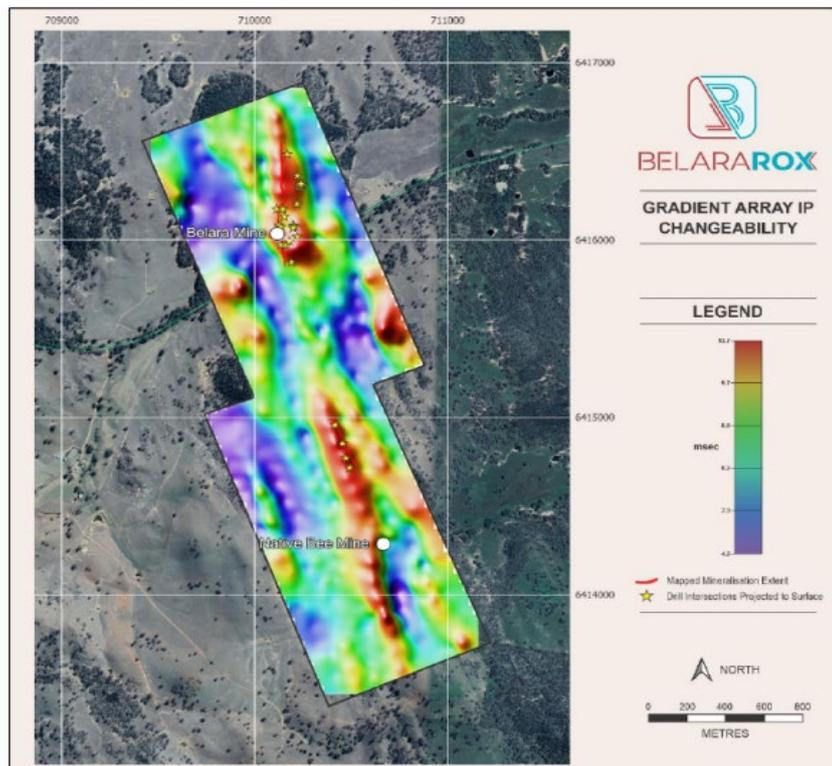
Figure 4. Gradient array IP chargeability data mapped in comparison to the extent of the known massive sulphide mineralisation and historic drill intersections (refer to ASX announcement dated 23 March 2022). The chargeability high values mapped in red correspond to the known massive sulphides and extend along strike from both mines
