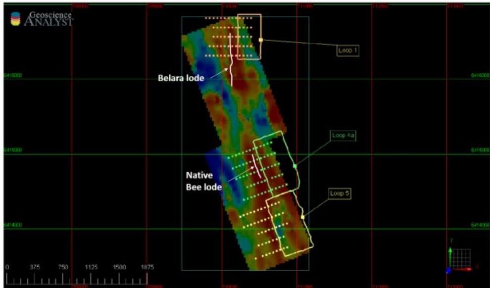
Figure 1. FLEM loop and stations at Belara and Native Bee. The background image is the gradient array chargeability response (refer to ASX announcement dated 23 March 2022). White polygons are the outline of the known mineralisation at 25m below surface
