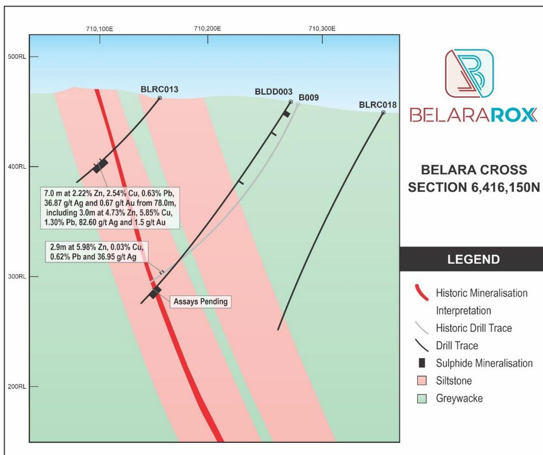
Figure 3. Section 6416150mN of drill intersection in BLRC013 relative to historic hole B009, interpreted geology and interpreted massive sulphide mineralisation from the historic model. Note BLRC018 will be completed using a diamond tail and the assays for BLD003 have not been finalised.
