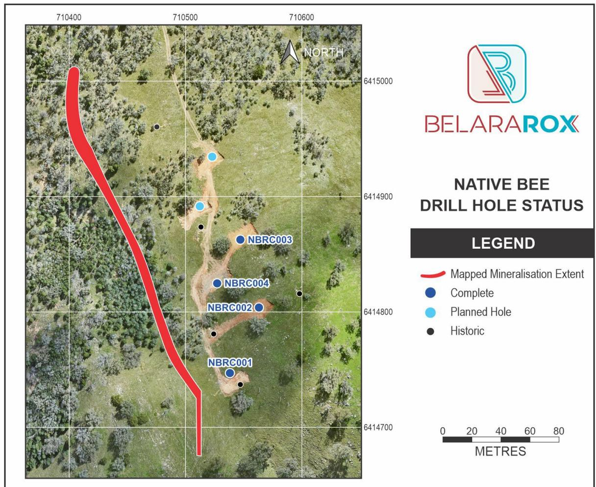
Figure 2. Drill location plan of resource definition holes at the Native Bee mine compared to the historic holes.
