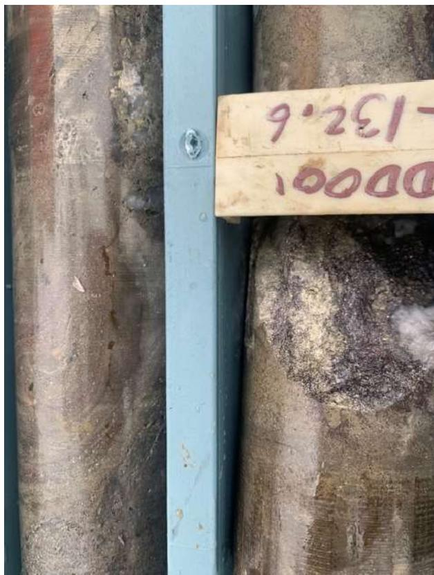
Figure 1. Zinc rich massive sulphide mineralisation at 132.6m.
