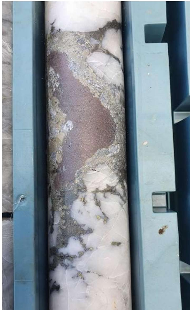
Figure 3. Hole 2: Zinc rich (pink sulphide) and copper rich (yellow sulphide) massive sulphide mineralisation at 168.13m which forms part of the 19m downhole intersection.
