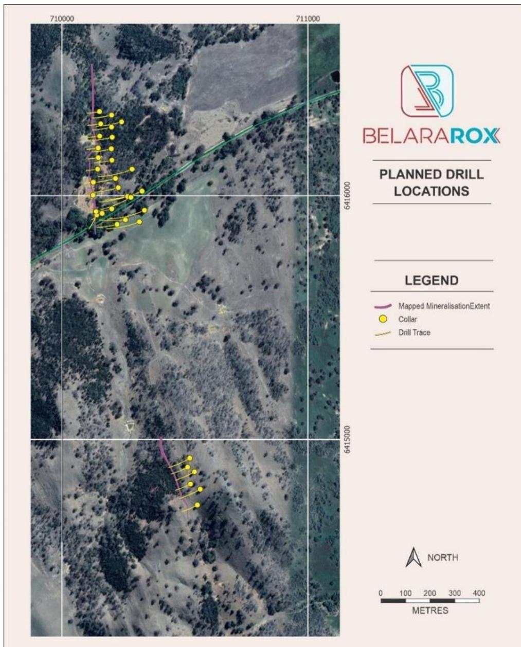
Figure 3. Drill location plan of planned resource definition holes at the Belara and Native Bee mines compared to the historic holes.
