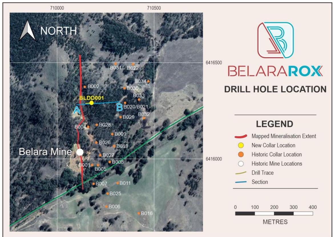
Figure 4. Drill collar location plan of drill collars at the Belara mine compared to interpreted massive sulphide mineralisation.
