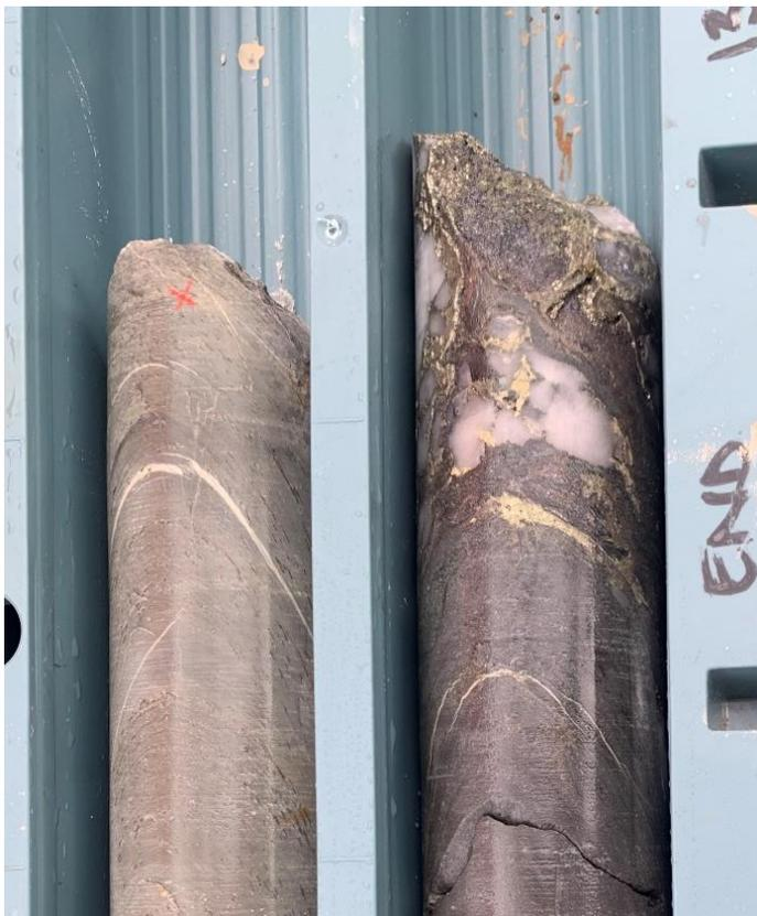
Figure 2. Copper rich massive sulphide mineralisation at 132.0m.
