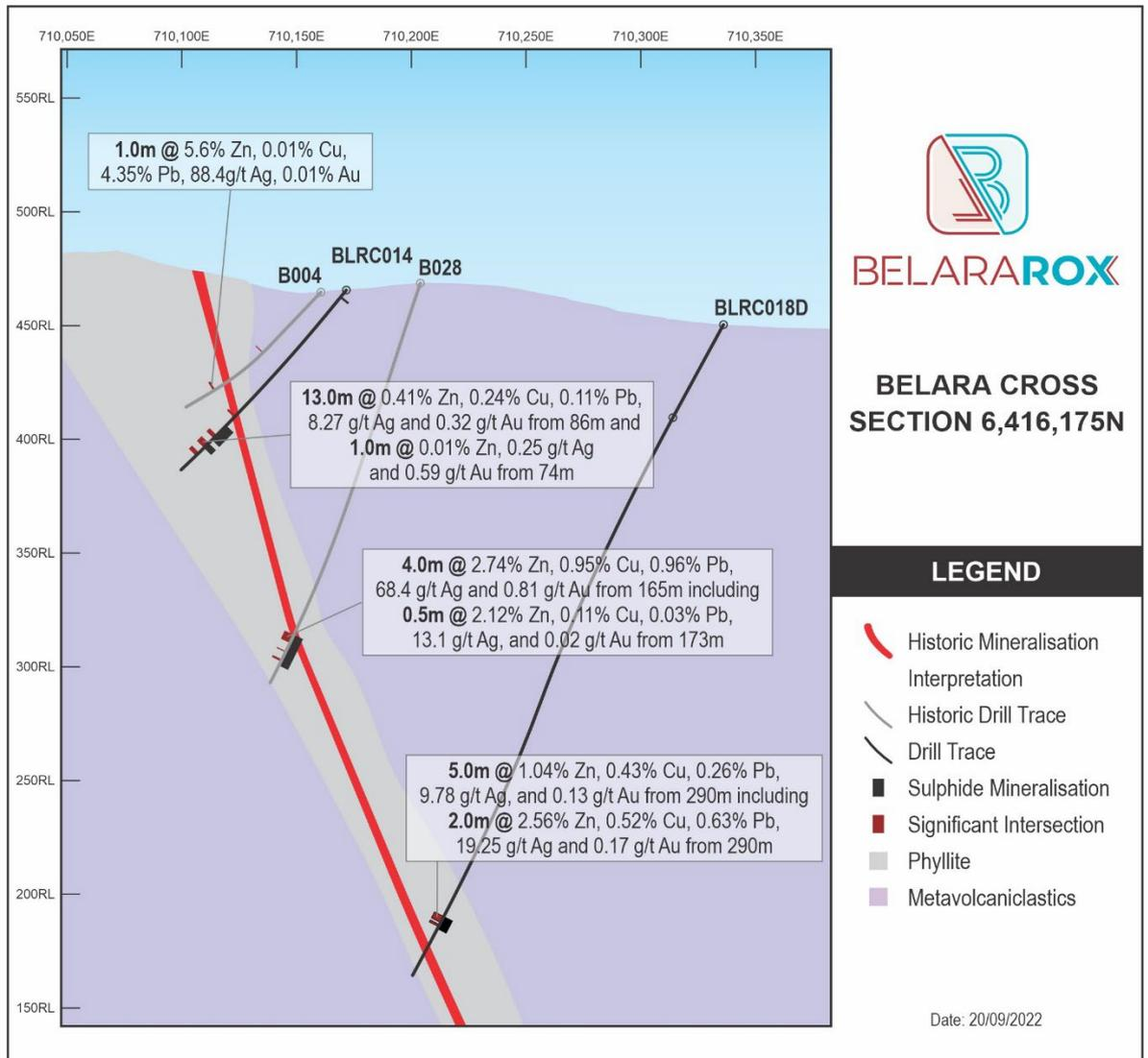
Figure 3. Section 6416175mN showing results from drill holes BLRC014 and BLRC018D relative to historic holes B004 and B028, interpreted geology and interpreted massive sulphide mineralisation from the historic resource.
