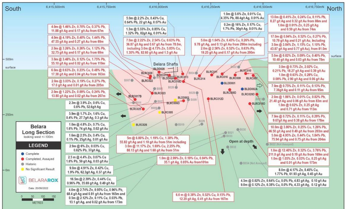
Figure 5. Long section (along the plane of mineralisation) showing significant intersection from new results and previous results from Phase One resource drilling at Belara and historical results.
