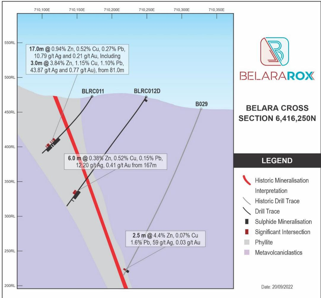
Figure 4. Section 6416250mN showing results from drill holes BLRC011 and BLRC012D relative to historic hole B029, interpreted geology and interpreted massive sulphide mineralisation from the historic resource.
