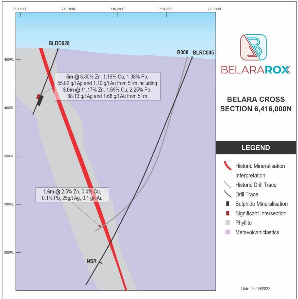
Figure 2. Section 6416000mN showing new results from BLDD028, interpreted geology and interpreted massive sulphide mineralisation from the historic resource. NSR stands for no significant results.
