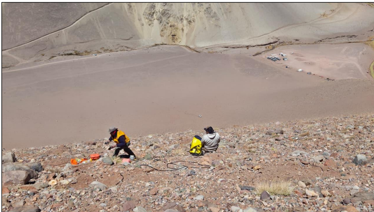
Figure 3: Quantec technicians laying out the MT/IP survey lines across the Toro targets. Note the TMT Camp in the top right corner for scale.
