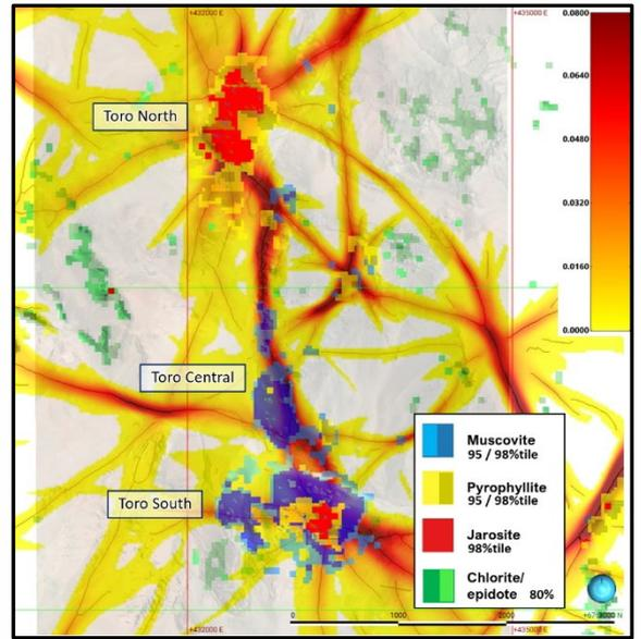
**Figure 3:** Linear zones of iron-oxide – kaolinite – phyllic alteration and the mineral models derived from the processing of ASTER and Sentinel-2 satellite spectral data in the Toro project. (Garwin, 2023; Core & Core, 2023)
