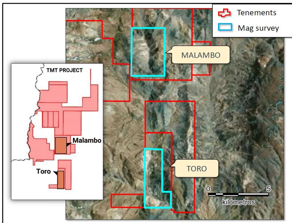
Figure 10: Planned Drone Magnetic Survey areas
