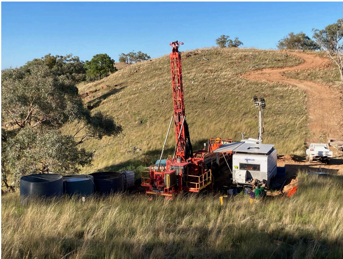
Figure 1. Sandvik DE712 diamond rig (Ophir Drilling) drilling the first Phase 2 drill hole at Native Bee.
