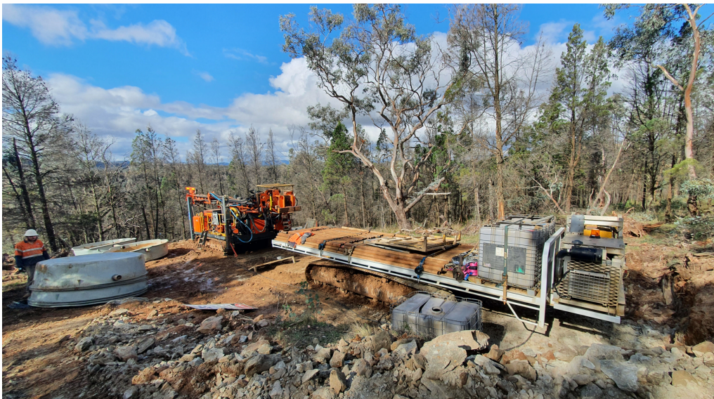
Diamond drill rig has arrived on site to diamond tail the RC pre-collars on the deeper resource holes.
