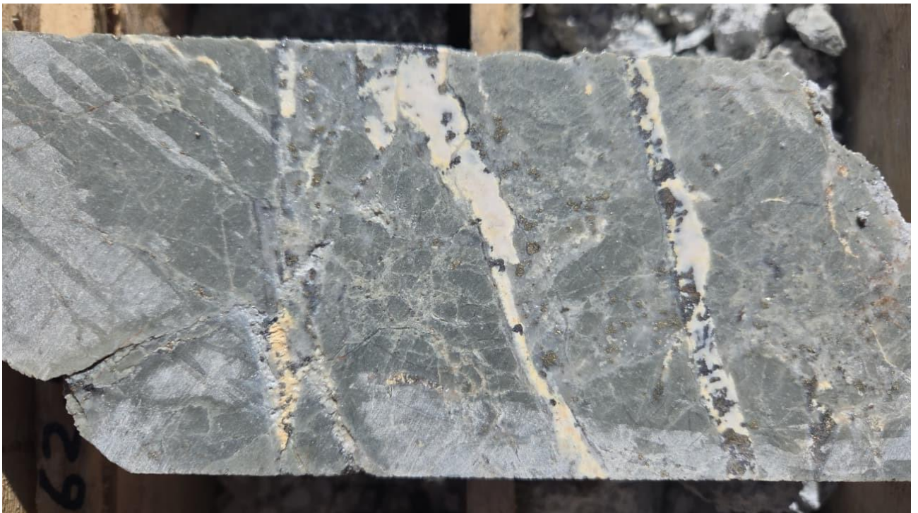
Figure 8. Drill core from TCDDH002 at 61.8m showing typical veining and sulphide mineralisation from the high grade intersection of 47m @ 171.99 g/t Ag, 3.99% Zn, 0.23% Cu, 0.22 g/t Au and 0.34% Pb from 59m.
