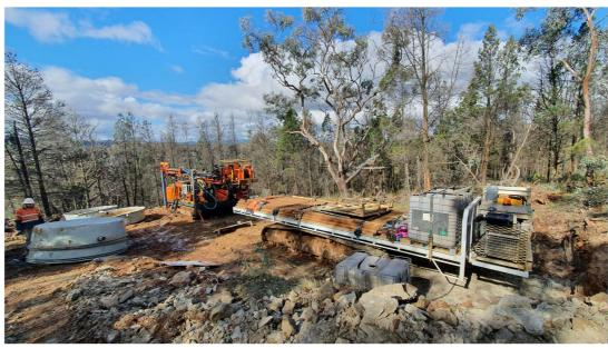
Diamond drill rig has arrived on site to diamond tail the RC pre-collars on the deeper resource holes.
