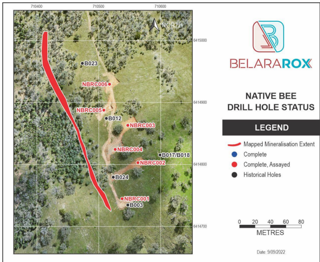
Figure 2. Drill location plan of resource definition holes at the Native Bee resource area compared to the historic holes
