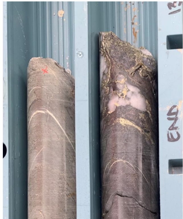
Figure 9. Copper rich massive sulphide mineralisation at 132.0m.
