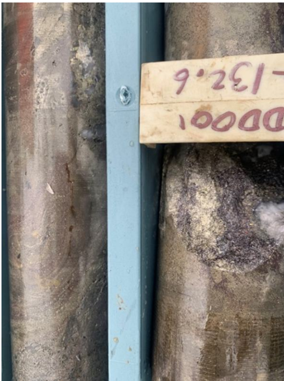
Figure 8. Zinc rich massive sulphide mineralisation at 132.6m.
